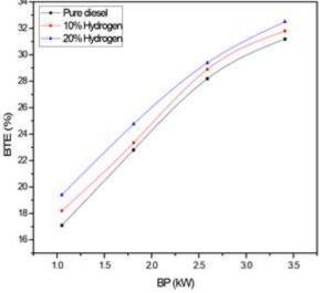
Fig. 3. Variation of brake thermal efficiency with Brake Power
