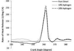
Fig. 9. Rate of heat release at different hydrogen substitutions.
