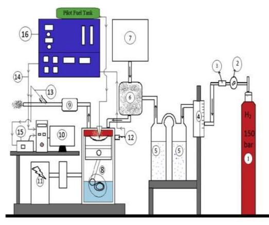
1.H<sub>2</sub> gas cylinder 2.Pressure gauge 3.Back flash arrestor 4.Flow meter 5.Flame arrestor 6.Mixing chamber 7.Air tank 8.Engine 9.Exhaust gas calorimeter 10.PC 11. Eddy current dynamometer 12.Piezoeletric sensor 13.Exhaust gas sensor 14. Sensor to PC 15.Exhaust anlyser 16.Control panel
