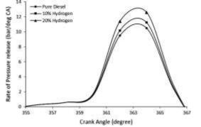
Fig. 10. Rate of pressure release at different hydrogen substitutions
